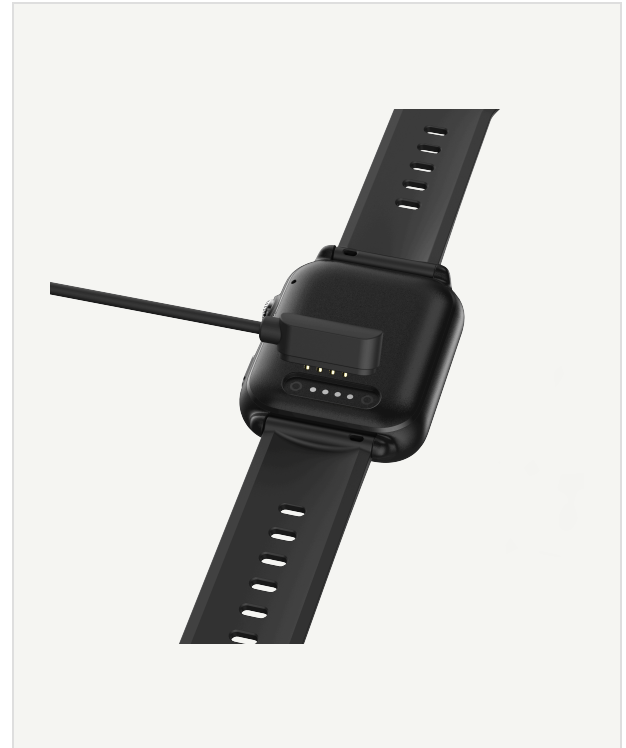
Align the magnetic charger so it sits flush.
